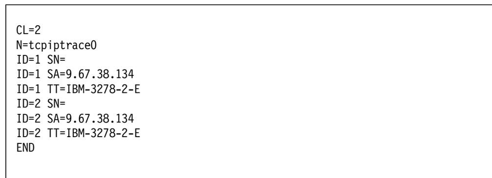
Figure 149. Telnet3270 Configuration File PC3270.TCP - DOS FF Mode
